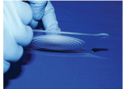
**Abrasive waterjets are frequently used to cut glass. With today’s control technology, tolerances of +/-0.001" are being achieved by Abrasive Waterjet & CNC.**
